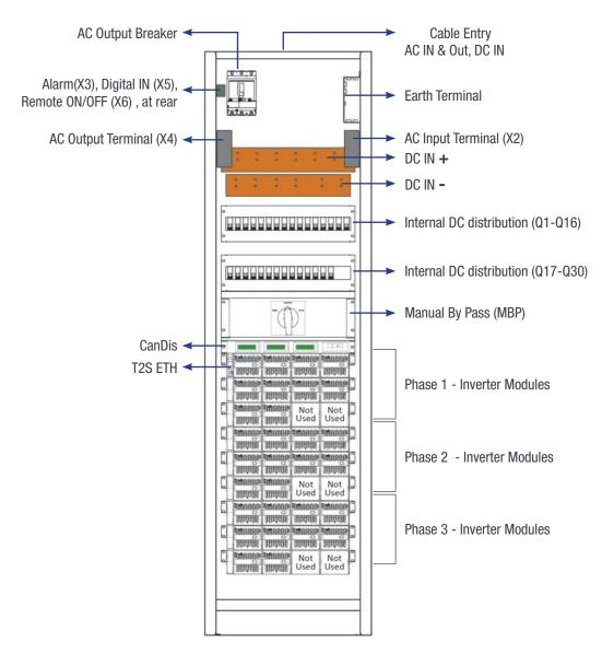
Bravo EQZ4 90 kVA Inverter System - General Arrangement
